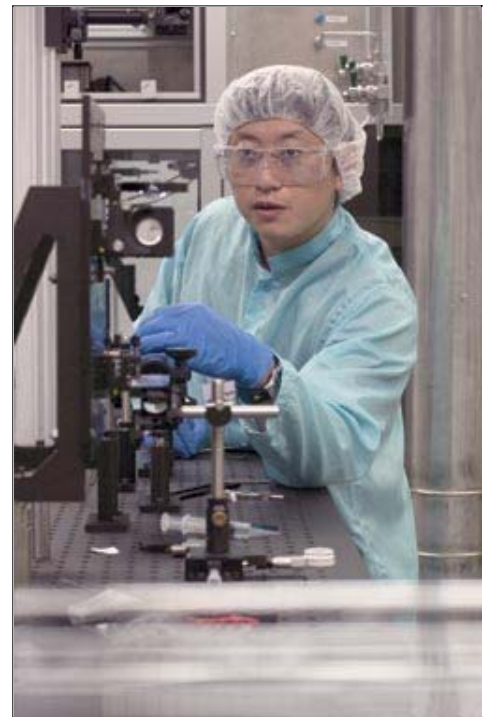
Researcher Jianming Zhou aligns the immersion lithographic system.
